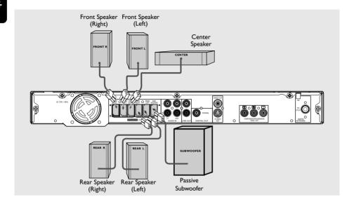
Connect the supplied speaker systems using the fixed speaker cables by matching the colors of the jacks and speaker cables.
